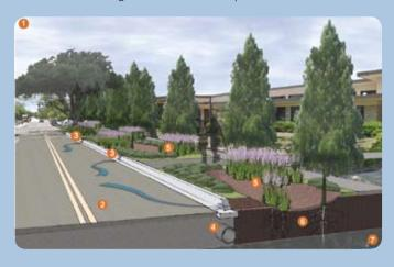
to traditional stormwater practices. A portion of the runoff from Lasalle Street and the surrounding area will now be diverted into the bioswale, helping to clean the stormwater before it enters our river.
